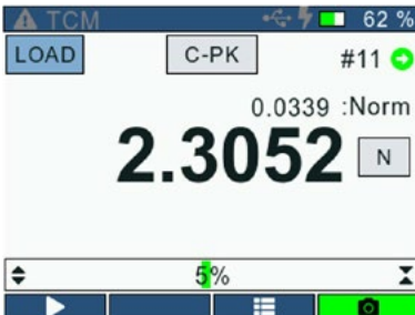
Live result screen with run number, pass/fail indicator, units, and display mode.
