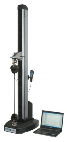
The LS2.5 is a 2.5 kN / 562 lbf high precision material testing machine that combined with our extensive ra  $\,$  nge of grips, fixtures, extensometers and software creates a powerful material testing system. The s  $\,$  ystem is equally suited to quality control, educational and R& D environments within a wide range of applications and test types. The system is particularly suited for plastic, rubber and other high elongation materials due to its wide crosshead travel capability.
