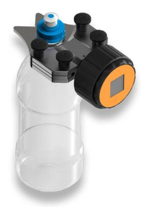
Continuous thinner packaging of noncarbonated beverages requires to stabilize the package by nitrogen injection after filling. If the packages are equipped with sports closures, that can't be pierced from the top, new instruments are required to assure the ideal inner pressure for most optimal performance of the package.
