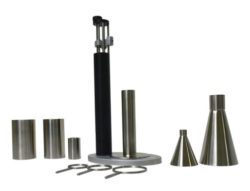
The device ADT-321 brand ATRYA, allows to perform the 3 methods described in the standard ASTM D 1895. According to the standard, "These test methods cover the measurement of apparent density, volume factor and, where appropriate, the pouring capacity of plastic materials such as molding powders". Test method A is equivalent to method ISO R 60 as described in the Appendix. This tester can be used in laboratory or within production lines to ensure raw material meet industry specifications.
